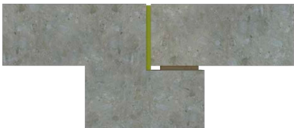
• Traditionele oplossing "halfhout"-verbinding
